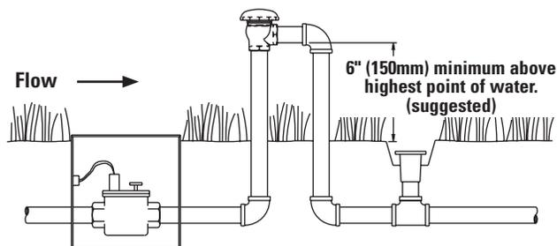
**NOTE:** Unit cannot have any shutoff downstream of it.
