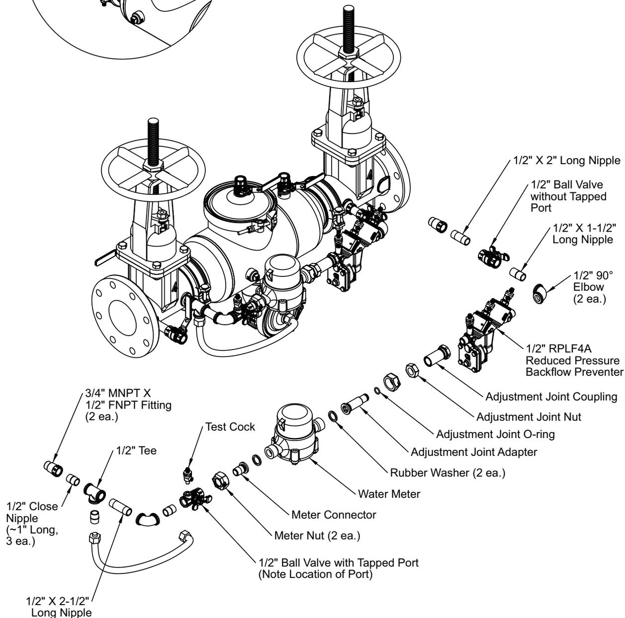
APPLY TEFLON TAPE TO PIPE THREADS AND INSTALL COMPONENTS AS SHOWN.
