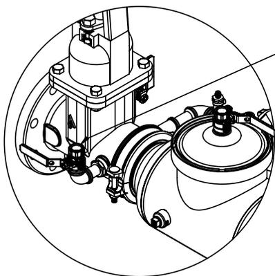
Note: Before attaching bypass line, remove #2 test cock, nipple, and reducer and move to the opposite side of the gate valve.
