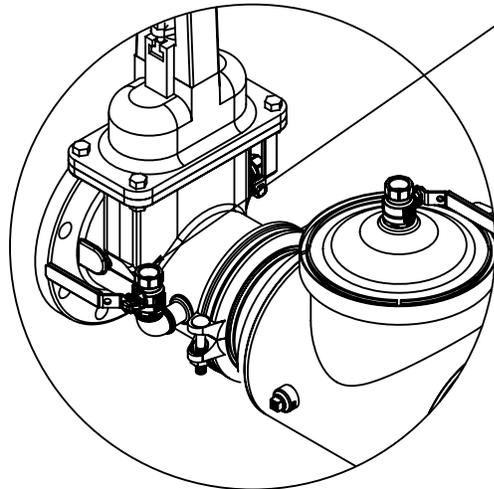
Note: Before attaching bypass line, remove #2 test cock and nipple and move them to the opposite side of the gate valve.
