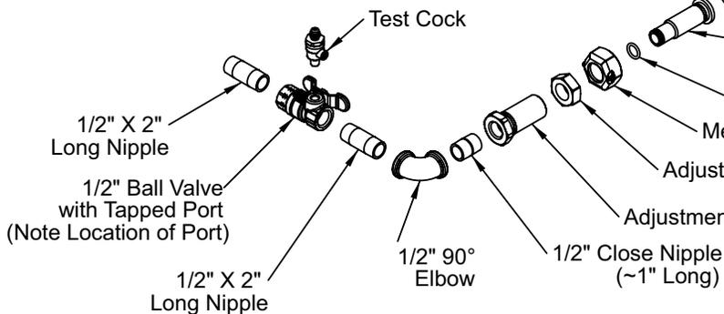
APPLY TEFLON TAPE TO PIPE THREADS AND INSTALL COMPONENTS AS SHOWN.
