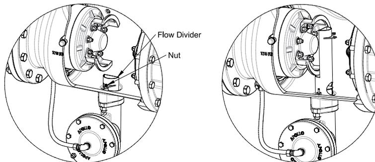
**NOTE:** On 10" & 12" models, the flow divider (FD) must be removed before the checks are removed. To remove the FD, remove the 1/4" nut holding it in place. Then rotate the FD 90° and lift up and out of the valve body. Pay attention to which side of the body the FD is attached. The FD's tab should be oriented on the same side as the cover of the relief valve body. If the relief valve needs to be turned 180°, the FD must also be rotated 180°.
