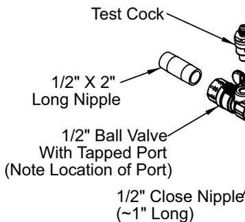
APPLY TEFLON TAPE TO PIPE THREADS AND INSTALL COMPONENTS AS SHOWN.
