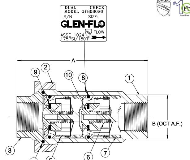
Max Temp 180°F (82°C) Max Pressure 175psi (12bar)
