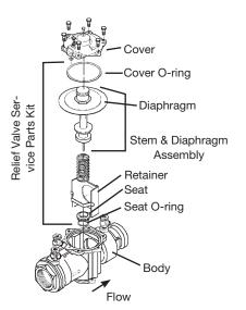
After initial installation, a discharge from the relief valve opening may occur until all sealing surfaces have become seated or due to inadequate initial flushing of pipe lines to eliminate dirt and pipe compounds. If flushing will not clear, remove the first check valve and clean thoroughly.
